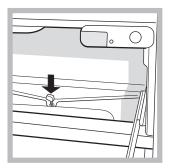
produced by the compressor causes it to evaporate. It is not, therefore, necessary to defrost the refrigerator manually. It is, however, necessary to clean the discharge hole regularly so that the water can flow out easily.
